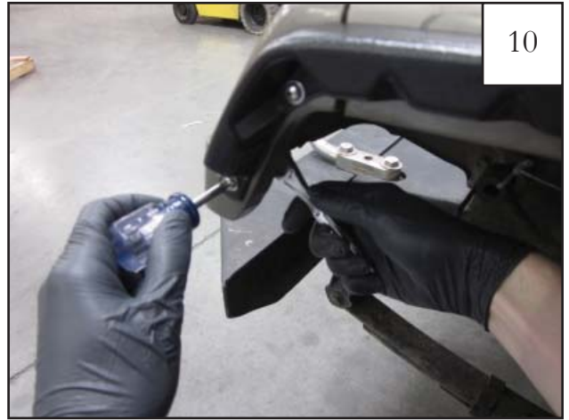
Step 3 Fully tighten Nuts (NU1-0010) using a 5/16" socket wrench and a # 2 Phillips bit for the Screws (SW1-0053).
