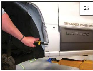
Use pliers to bend back horizontal sheet metal tabs. Use a hammer to flatten out sheet metal tabs. Avoid bending or distorting outer sheet metal.
