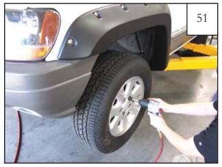
Re-install tire using an impact wrench.
