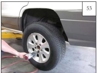
Remove tire using an impact wrench.
