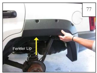
Hold assembled flare in place on vehicle aligning forward edge with the door seam and inside edge of rear main part with fender lip. Confirm fit cut areas and make adjustments as needed.
