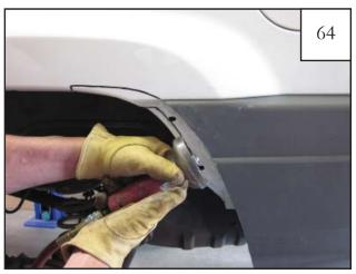
Using a cut off wheel or other suitable tool, cut along line marked in step 63 removing the inner flange.
