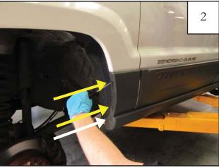
Using a #2 Phillips Screwdriver, remove factory screws from upper side cladding (2 places). For models with rocker panels installed, remove screw from end of rocker panel (1 place).
