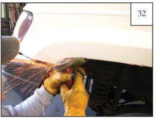
Starting at the front edge, cut out mark shown in Step 20.
