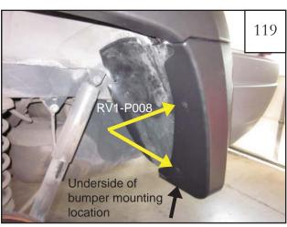
Install three panel retainers (RV1-P008) through flare and into mounting brackets and underside of bumper mounting location as shown.
