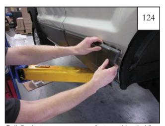
Pull firmly to remove upper factory side cladding piece from fender.
