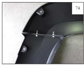
Using a 7/16" wrench and 3/8" socket, bolt rear main flare to bumper piece using supplied screws (SW1-0006) and nuts (NU1-0011). Do not fully tighten screws. Parts are marked on the inside. Driver's side: D3 for main flare, D4 for bumper piece. *Note: Be sure to select the correct style bumper.*
