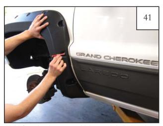
Hold flare in place on vehicle, mark hole locations on fender through holes drilled in pockets of flare.
