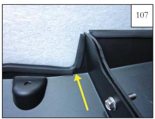
The Edge Trim (GP1-0005) on the sharp inside radius of bumper piece may need to be notched to fit correctly.
