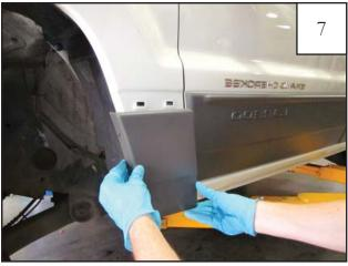
Pull firmly to remove upper factory fasteners in front side cladding piece from fender. Clean exposed sheet metal.
