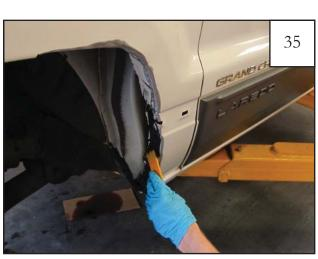
Apply urethane caulking or primer to seal any exposed sheet metal for rust prevention.
