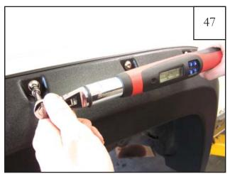
With the edge trim in place and once all screws have been started, snug screws to vehicle. Torque screws to 24 in•lb (2 ft•lb). DO NOT OVERTIGHTEN!
