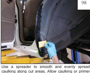
Use a spreader to smooth and evenly spread caulking along cut areas. Allow caulking or primer to partly dry before proceeding. Does not need to be fully cured.
