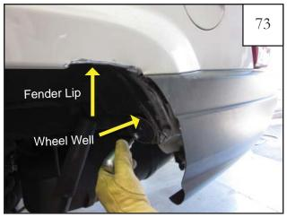
Using an angle grinder or sandpaper, sand the chipped paint along bent edges of the fender lip and wheel well.
