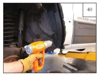
Using a heat gun, heat splash shield until pliable and use heavy work gloves to push and mold splash shield into place aligning with trimmed inner wheel well. Hold it in place and allow to cool. Then fully install push retainers in splash shield.
