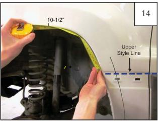
Starting at upper style line, measure up 10-1/2" from upper style line of cladding/sheet metal along edge of wheel well and mark with grease pencil.
