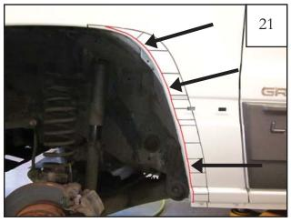
Make a mark approximately 1/4" in from the edge of the wheel well lip starting at the bottom of the wheel well extending to the uppermost point of the markings.
