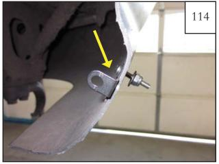
Start a washer (WA1-0014), screw (SW1-0054) and nut (NU1-0004) combination through the holes and brackets in bumper. Use a washer for both screw head and nut. The bracket should face inward and the screw head should be on the inside if of the bumper.
