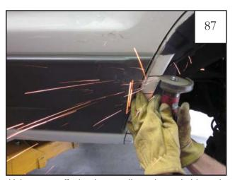
Using a cut off wheel, sawsall or other suitable tool, cut along horizontal marks from wheel well to vertical line. **NOTE: DO NOT OVERCUT!**
