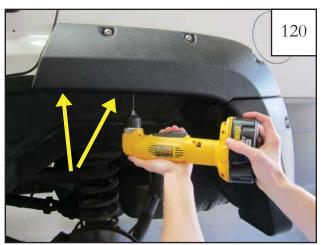
Predrill fender lip at top horizontal area with a 1/8" drill bit through holes in rear main flare (2 places).
