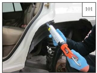
Prior to installation of the cut cover, apply another layer of caulking to help keep cut cover in place.
