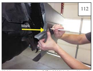
Hold mounting bracket (MB1-0003) in line with mark made in step 111 and make a mark through the hole location in the bracket. Repeat for second bracket.
