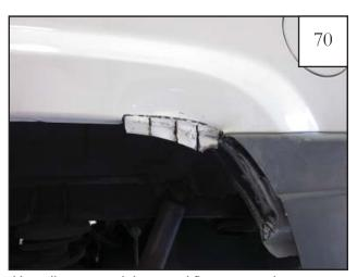
Use pliers to straighten and flatten out tabs. Note: May need to cut away additional portion of tab on the radius to allow room to flatten tab to inner wheel well.
