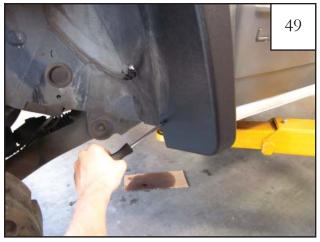
Using a phillips screwdriver, install supplied screw (SW1-0056) into hole drilled in step 47.
