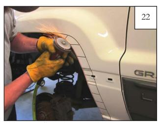
Using a cut off wheel or other suitable tool, cut along line marked in step 21 removing the inner flange.
