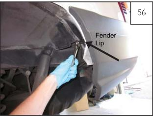
Using a 10mm deep socket and wrench, remove bolts on inner side of fender lip (2 locations).
