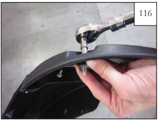
Put screw (SW1-0045) through holes in pockets of rear main flare and bumper piece and secure with rubber grommet (SP1-0009) using supplied #45 Torx bit (SW1-0052). Drive screw into grommet until tight. Repeat for all pockets.
