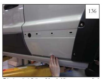
Prior to re-installation of the cladding, use a supplied alcohol prep pad to clean the sheet metal and any factory tape residue.
