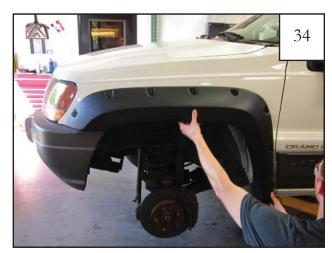
Hold flare up to wheel well to confirm fit. Make adjustments to cut as needed.
