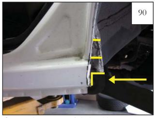
Cut away lower corner of pinch weld.
