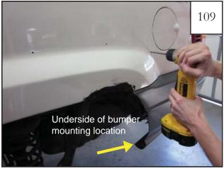
Drill holes in fender and bumper at marks with a 3/16" drill bit. Use 1/4" drill bit to drill mark on underside of bumper.
