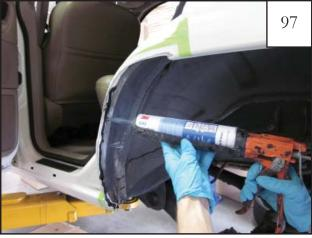
Apply urethane caulking or primer to all cut areas of wheel well to seal any exposed sheet metal for rust prevention.
