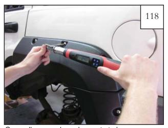
Once all screws have been started, snug screws to vehicle. Torque to 24 in•lb (2 ft•lb). DO NOT OVERTIGHTEN!
