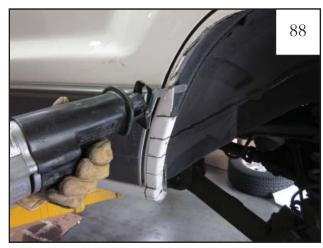
Using a cut off wheel, reciprocating saw or other suitable tool, remove tabs cut in previous step. Tip: Using a reciprocating saw works best for this cut. **NOTE: DO NOT OVERCUT!**
