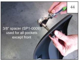
For all remaining pockets, install a #45 Torx screw (SW1-0045) through pocket hole and secure with rubber spacer (SP1-0009) using supplied #45 Torx bit (SW1-0052). Drive screw into spacer until tight. Repeat for all remaining pockets.
