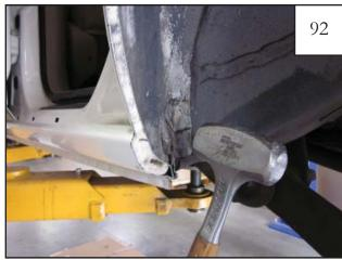
Using a hammer, flatten pinch weld tabs against inner wheel well.
