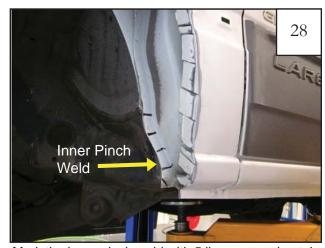
Mark the inner pinch weld with 5 lines approximately 2 inches apart starting from the bottom.
