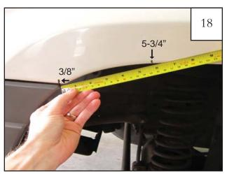
Where the bumper and fender meet along inner wheel well, make a mark 3/8" in from wheel well. Then measure back 5-3/4" along edge of fender and mark.
