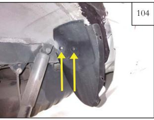
Re-install splash shield using supplied panel retainers (RV1-P008). **NOTE: Do not fully install push retainers. Splash shield must be re-molded. See step 105.**
