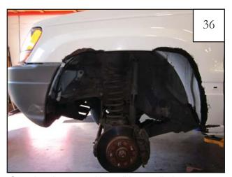
Completed cut-out with caulking applied.
