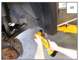
Using a 3/32" drill bit, drill hole through flare into sheet metal near the back inside edge of the wheel well.
