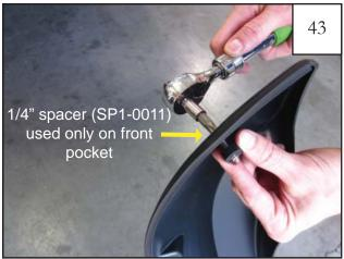
Install a Torx screw (SW1-0045) through <u>FRONT</u> pocket hole of flare and secure with rubber spacer (SP1-0011) using supplied #45 Torx bit (SW1-0052). The torx bit fits into a 5/16" socket. Use with a 3-6" extension for drill or air ratchet. Drive screw into spacer until tight.
