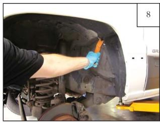
Using a pry tool or utility knife, remove factory fasteners from wheel well splash shield (9 places).
