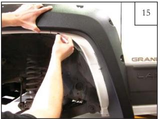
Hold the flare up to the fender as a guide. Make a line connecting the marks made in steps 13 & 14.
