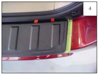
Hold the part at an angle to prevent tape from prematurely sticking, and align the part on the bumper by centering bump in rear door sill between two center ribs in part and using the masking tape applied in Step 1 as a guide.
