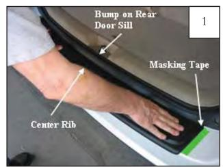
Open rear door of vehicle. WITHOUT peeling liner, align part on bumper, centering the center rib of the bumper guard with metal loop on striker. Apply a piece of masking tape along both edges of part for ease of placement during installation.
