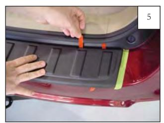
Maintaining part placement, stick peeled end to bumper and begin pulling center tab. Continue pulling center tab while applying pressure. Repeat process for liner the front of the vehicle, and the liner towards the back of the vehicle.
