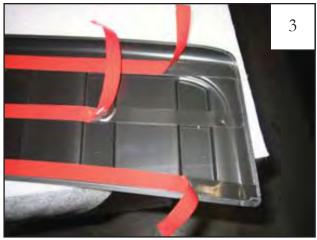
Peel the red plastic liner from the tape strips located on the inside of the bumper protector. NOTE: Make sure tabs are folded toward the outside of the part and that the middle tape liner is in front of rear liner.
