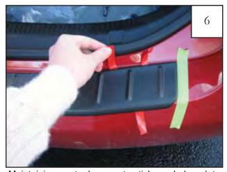
Maintaining part placement, stick peeled end to bumper and pull tab nearest the rear of the vehicle while applying downward pressure to rear edge of part. Repeat process for liner for center tape, then liner towards the front of the vehicle.
