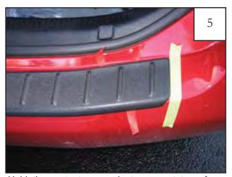
Hold the part at an angle to prevent tape from prematurely sticking, and align the part on the bumper by aligning center rib in part with metal loop on striker and using the masking tape applied in Step 2 as a guide.
