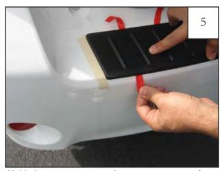
Hold the part at an angle to prevent tape from prematurely sticking and align the part on bumper by aligning shorter center rib in part with center of striker latch location and using the masking tape applied in Step 2 as a guide. Stick peeled end to Bumper and pull tab nearest the rear of the vehicle while applying downward/forward pressure to the rear edge of part.
