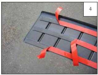
Peel red liners partially from tape pads. Center liner must be peeled back further or it will stick to outer liner tape pad. NOTE: Make sure tabs are folded toward the outside of the part.
