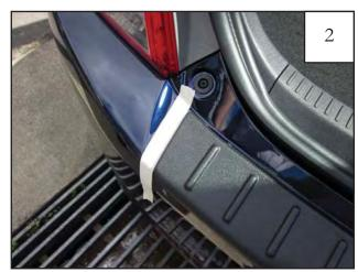
Apply a piece of masking tape along the driver side edge of part for ease of placement during installation.
