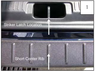
Open trunk of vehicle. WITHOUT peeling liner from tape pads, align part on bumper, centering the center, shorter rib of the bumper protector with the center of the striker latch location.
