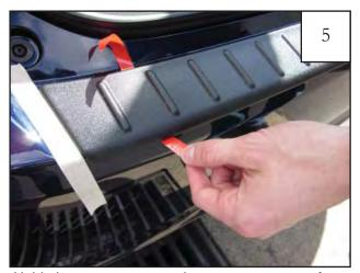
Hold the part at an angle to prevent tape from prematurely sticking and align the part on Bumper by center, shorter rib in part with center of striker latch location and using the masking tape applied in Step 2 as a guide. Stick peeled end to Bumper and pull red tab nearest the rear of the vehicle while applying downward/forward pressure to the rear edge of part.
