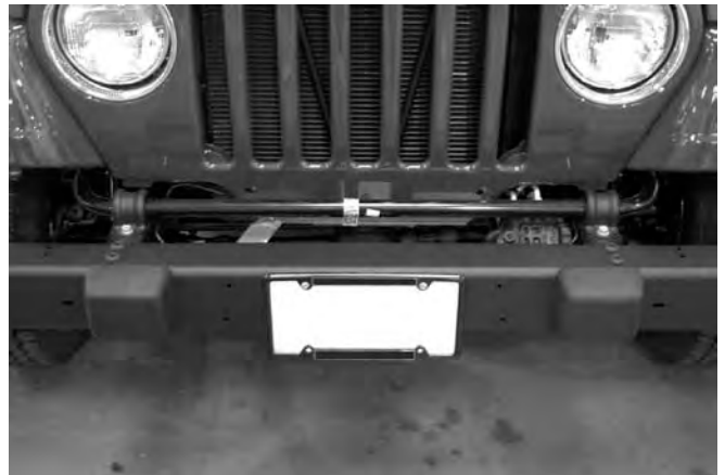
Figure #8 – Factory Front Panel Removed
