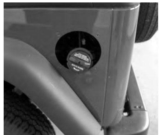
Figure #1 – Remove Gas Tank Outer Flange
