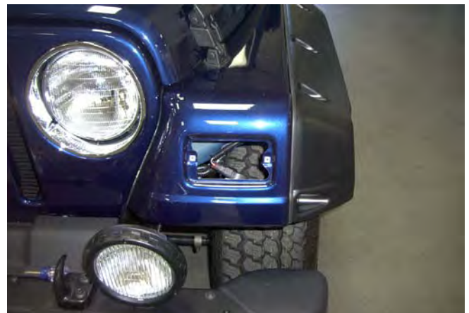
Photo #1 – Front Marker Light Cover Removed
