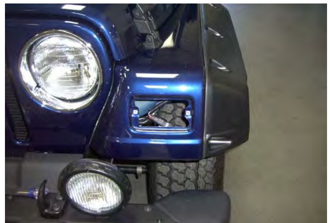
Photo #1 – Front Marker Light Cover Removed
