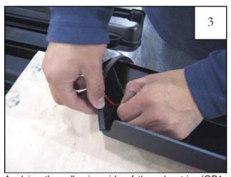
Applying the adhesive side of the edge trim (GP1-0005) to the inner side of part, affix edge trim to the top edge of the part (the portion that comes in contact with vehicle).
