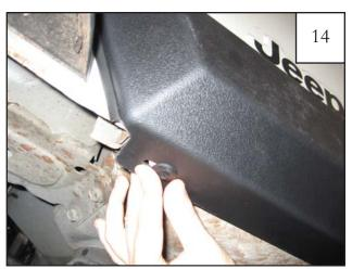
Attach underside edge of the Rocker Panel to the vehicle using supplied Tuflocs fasteners (RV1-P001), pressing Tuflocs through slots and into factory holes.
