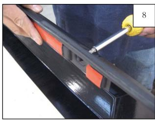
Using supplied Torx bit (SW1-0022), start a screw/ washer (SW1-0032 / WA1-0007) through each pocket into the indent in the inner piece (4-5 turns). Do NOT tighten!
