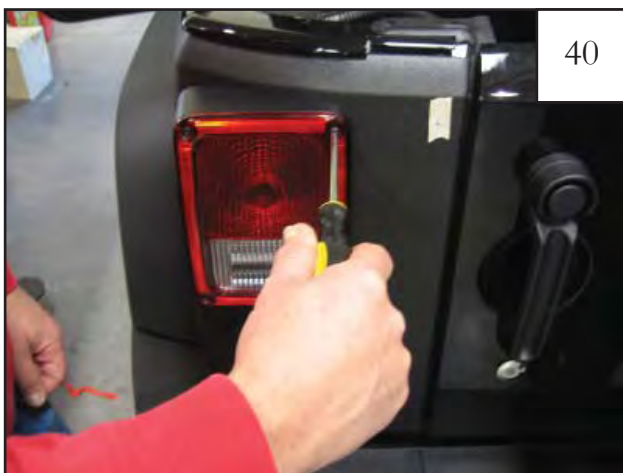
Using a #2 Phillips screwdriver, reinstall tail light.
