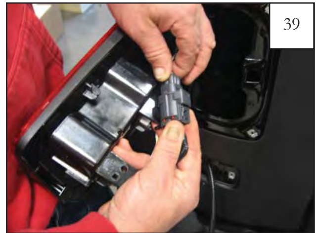
Reconnect light connector of tail light.
