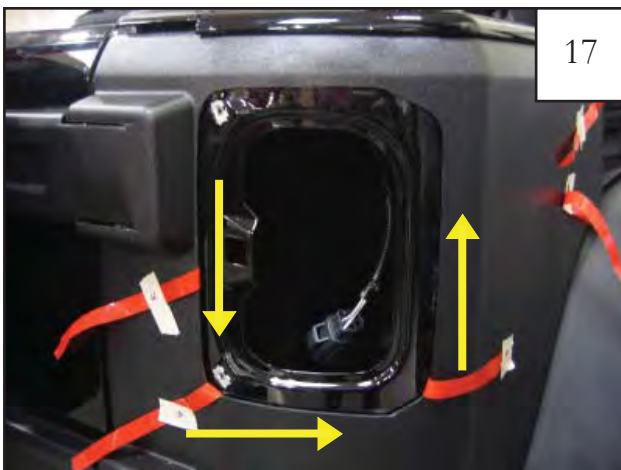
Tape liners 4, 5, & 6 may be removed in any order. Pull tape liner 4 downward. Pull tape liner 5 to the right. Pull tape liner 6 upward. NOTE: Refer to steps 8 & 9 for tape liner tab numbering.
