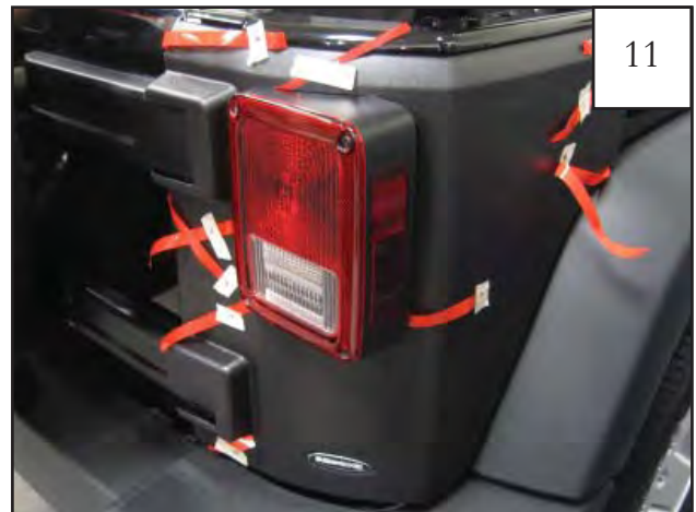
Make any necessary adjustments to the part to ensure it aligns properly around the tail light.
