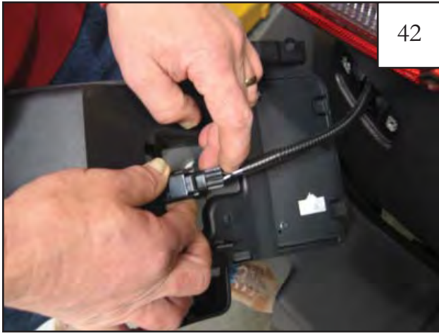
Reconnect light of license plate frame.
