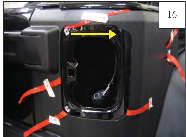
Pull tape liner 3 to the right toward the passenger side of the vehicle. NOTE: Refer to steps 8 & 9 for tape liner tab numbering.
