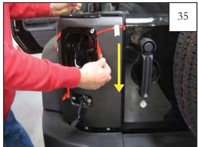
Pull tape liner 8 downward. NOTE: Refer to step 24 for tape liner tab numbering.
