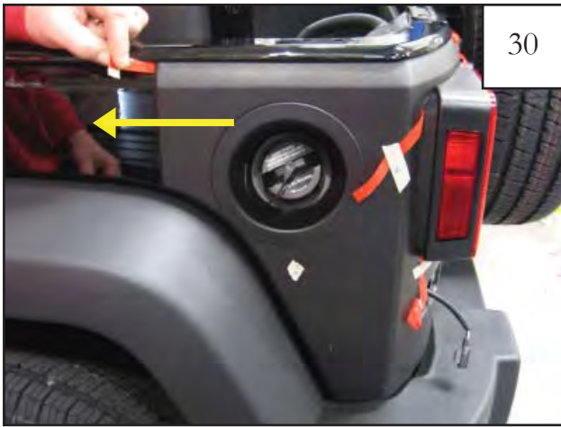
Pull tape liner 5 left toward the front of the vehicle. Press side of part firmly for proper tape adhesion. NOTE: Refer to step 24 for tape liner tab numbering.
