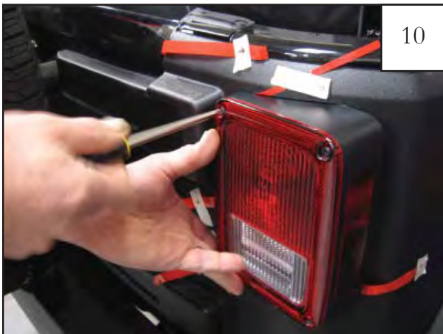
Position part on vehicle and using a #2 Phillips screwdriver, loosely start screws in the two locations they were removed from in the tail light.
