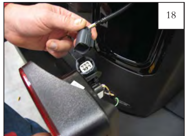
Plug the light connector back into the tail light and reinstall tail light using a #2 Phillips screwdriver.
