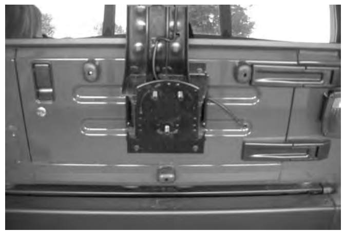
Figure #3 – Remove Spare Tire
