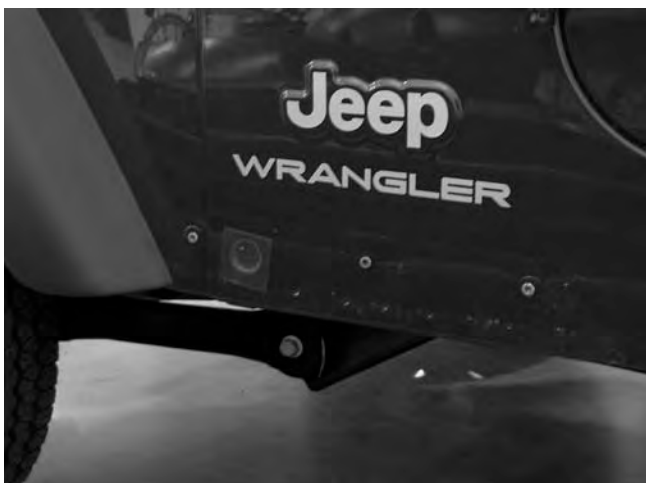
Figure #6 – Remove Stone Guard
