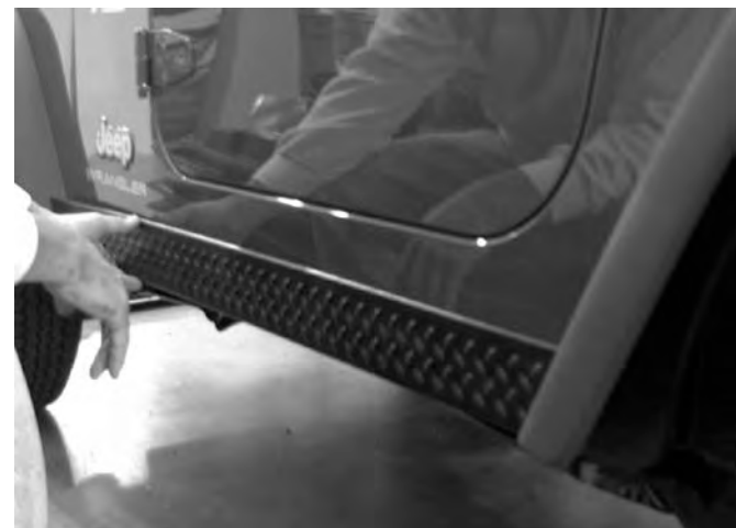
Figure #7 – Install Side Panel
