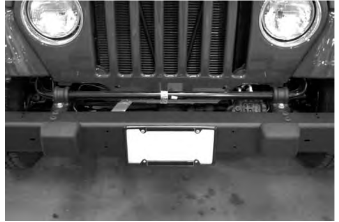
Figure #8 – Factory Front Panel Removed
