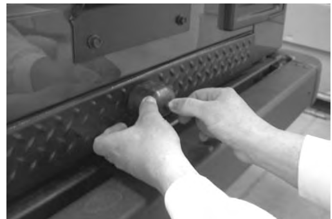
Figure #5 – Reinstall Tire Stop & Tire
