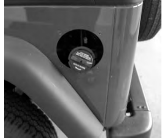
Figure #1 – Remove Gas Tank Outer Flange
