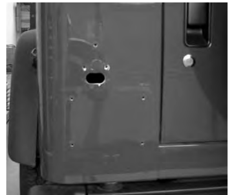
Figure #2 – Remove Tail Light & License Plate
