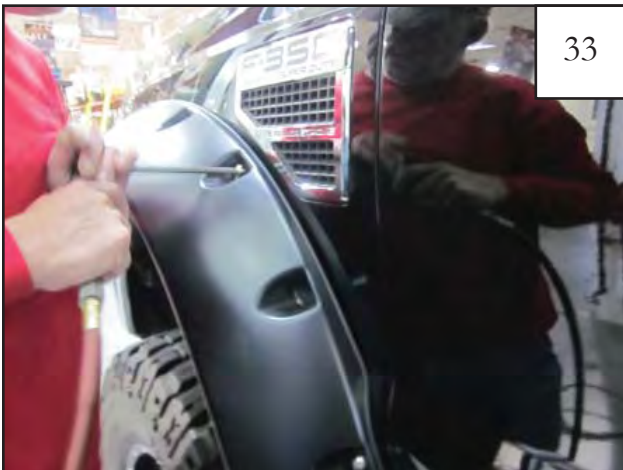
Using torx bit (SW1-0052), start bolts installed in Step 31 through holes drilled in Step 28. Once all bolts are in place, tighten all screws.
