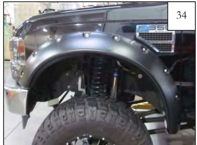
Completed front flare installation.
