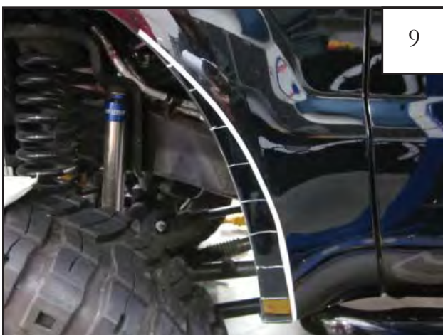
Mark fender with grease pencil about every 2" up to edge of masking tape.
