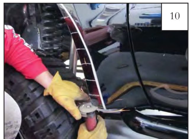
Using a cut-off wheel, cut fender along marked lines up to inner edge of tape.
