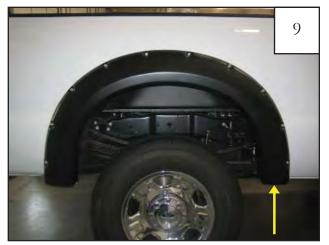
Place flare on fender and reinstall bolt removed in Step 4.
