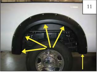
Ensuring proper flare placement, tighten all screws.
