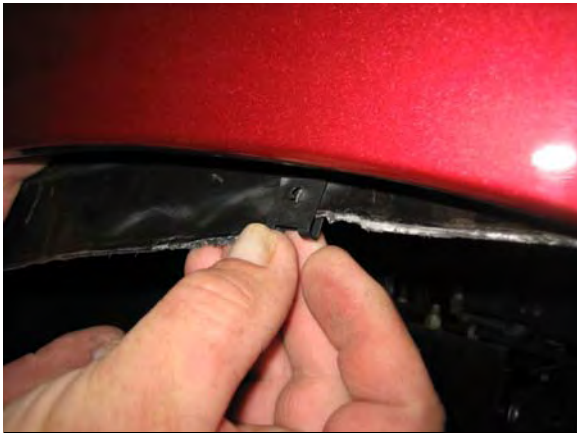
Photo #1 – Pull splash shield from behind fender. Install a supplied “U” Clip on splash shield as shown.
