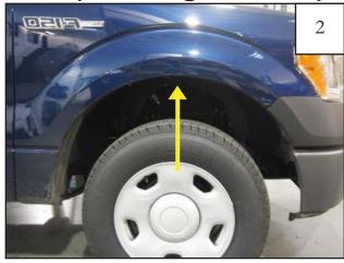
Install speed clip (CL1-0011) over fender wheel well lip. See step 3.
