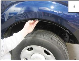
Line up the holes in the inner piece with the two uppermost factory holes and the speed clip. NOTE: Driver's side inner piece is marked with an "L" and passenger's side inner piece is marked with an "R".
