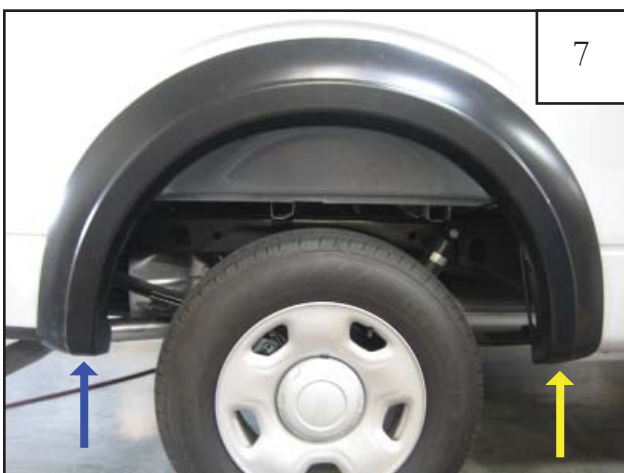
7 Using a 10mm socket wrench, tighten 35mm bolt through spacer and factory hole in sheet metal.
