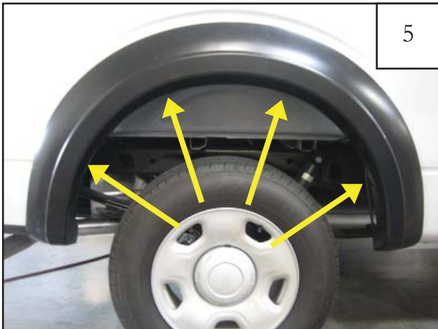
5 Hold flare to vehicle and start supplied truss head screws (SW1-0058) through the two topmost holes in wheel well. Then start supplied truss head screws (SW1-0058) through remaining two holes in flare. Tighten all screws.
