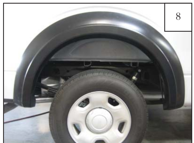
8 Completed rear flare installation.
