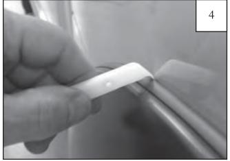
Using supplied Edge Trim Tool, seat edge trim against vehicle by hooking curved end under edge trim at one end of flare. Next, slide around outer edge of flare to the other end.
