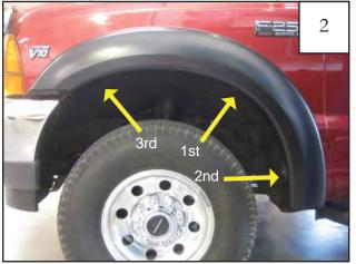
Position flare on fender and reinstall factory screws through holes in flare and fender with a 7/32" socket wrench in order shown. *NOTE: If given order is not used, part is more difficult to install.*
