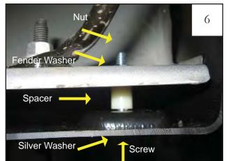
Start bolt from the bottom through a silver washer and into flare. Install spacer between flare and sheet metal. Slide a fender washer then the nut over the end of the screw.
