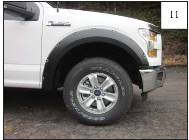
Completed front flare installation.
