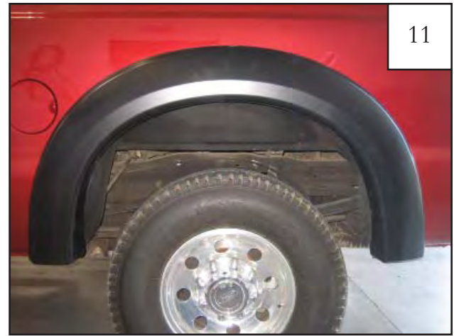
Completed rear flare installation.
