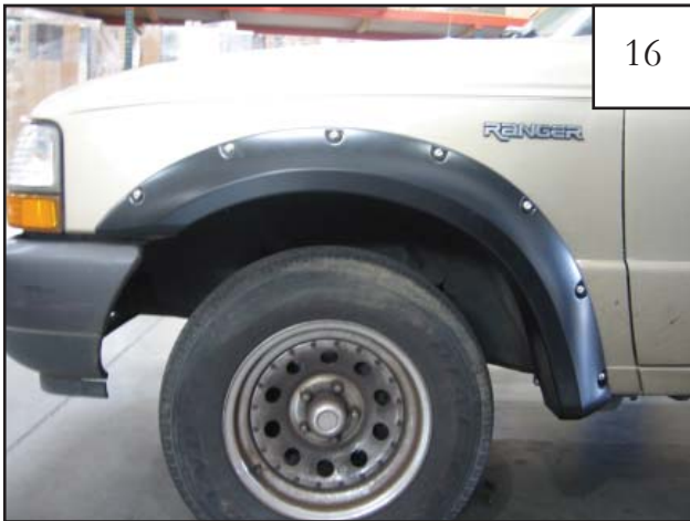
Completed front flare installation.
