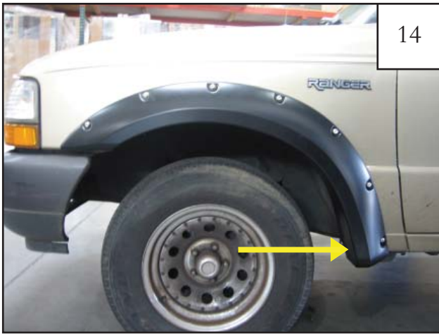
Reinstall factory screw saved from Step 8.
