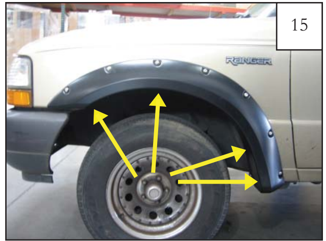
Ensuring proper flare placement, tighten all screws.
