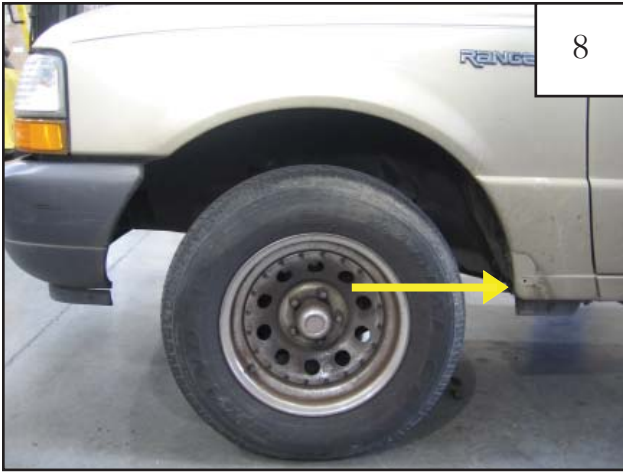
Remove factory screw at rear of wheel well. Save for reinstallation.
