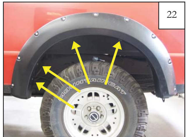
Reposition flare on fender ensuring that fender brace bolt is through lowest rearward hole and, starting with the rearmost wheel well hole, start Screws (SW1-0050) through holes in flare and into Clips (CL1-0022) with a #2 Phillips screwdriver.
