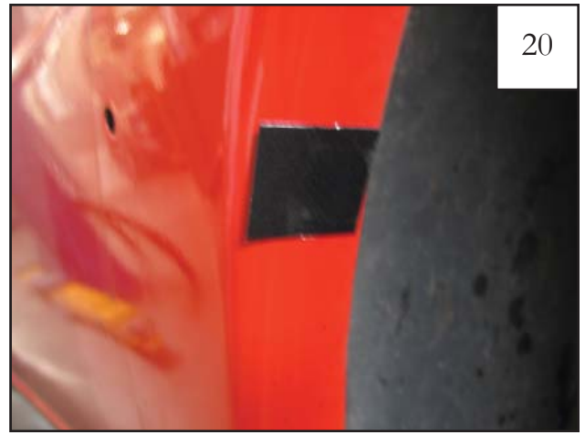
Install a Tab (MT1-0002) centered over each of the four holes marked in Step 19. Edge of Tab should be even with edge of sheet metal.
