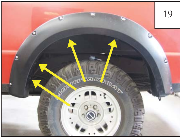
Mark through all flare holes using a grease pencil. Remove Flare.
