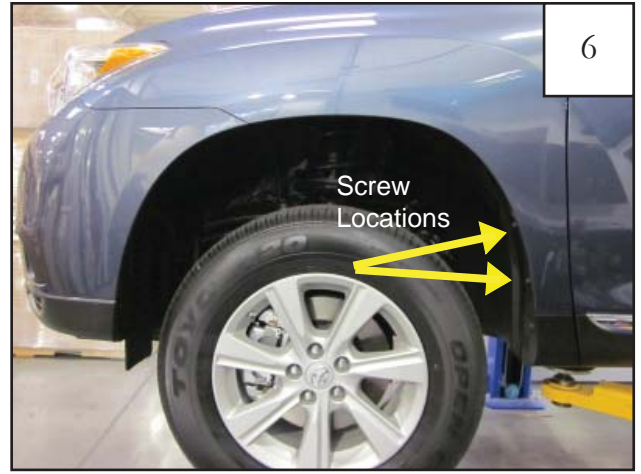
Two factory screw locations.
