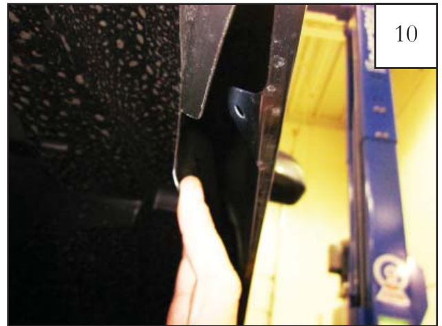
Pull wheel well liner out from behind fender lip.
