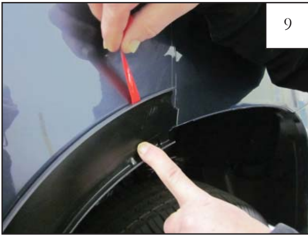
Pull remaining red tape liner and press the Inner Door Piece firmly to ensure proper tape adhesion.
