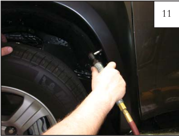
Start Screw (SW1-0036) through the one lower rear hole in flare and into factory hole in lower rear of wheel well.
