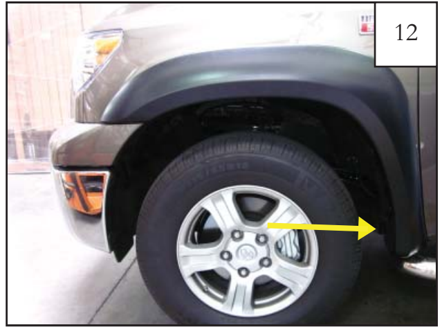
Screw (SW1-0036) lower rear wheel well location.
