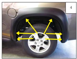
Hold flare firmly on the fender. Start a supplied Screw (SW1-0036) through each hole in flare and into hole in fender. (6 locations)
