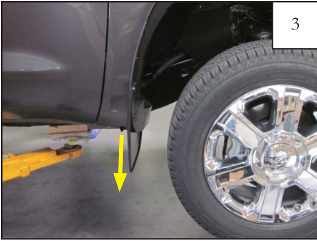
Remove factory push retainer from underside of factory mud guard. Remove mud guard from vehicle.
