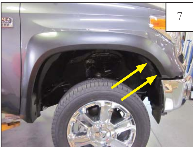
Start two supplied 20mm Hex Screws through forward most holes in flare and into factory hole locations.
