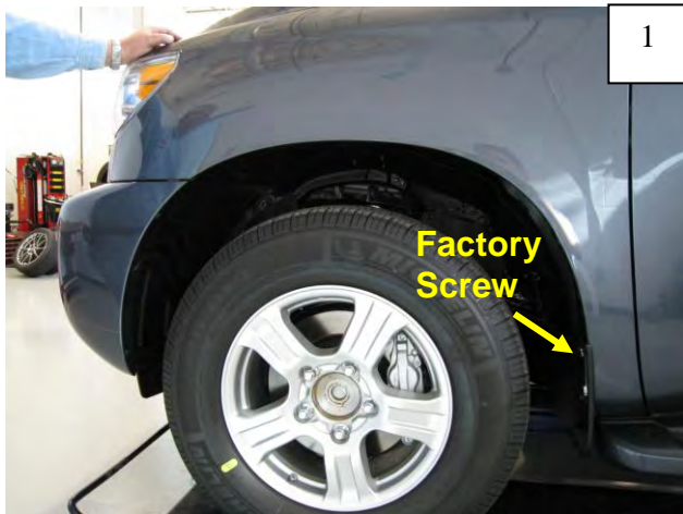
Remove one factory screw located at rear of front wheel well. Discard.
