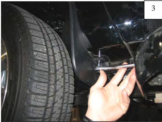
Remove one factory screw located at rear of mud flap area (under rocker). Discard.
