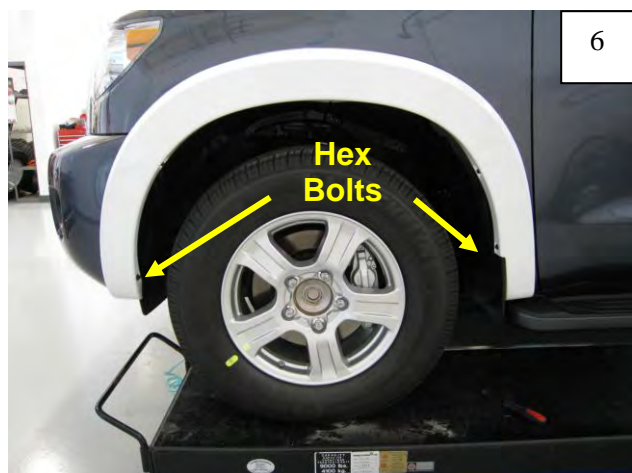
Position Front Flare on fender. Hand start supplied Hex Bolts through flare and into hole locations shown. Do not tighten.
