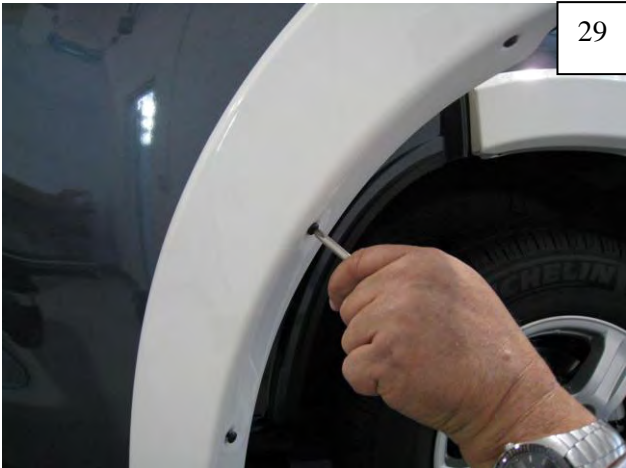
Start four supplied Door Screws. Do not tighten.
