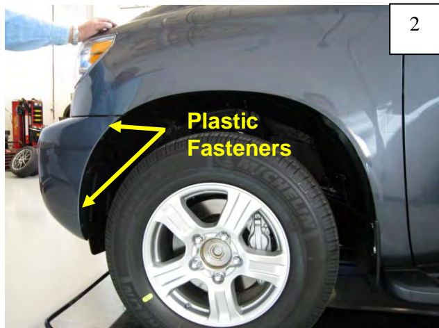
Use a trim tool or flathead screwdriver to remove two factory plastic fasteners located at front of front wheel well. Discard.
