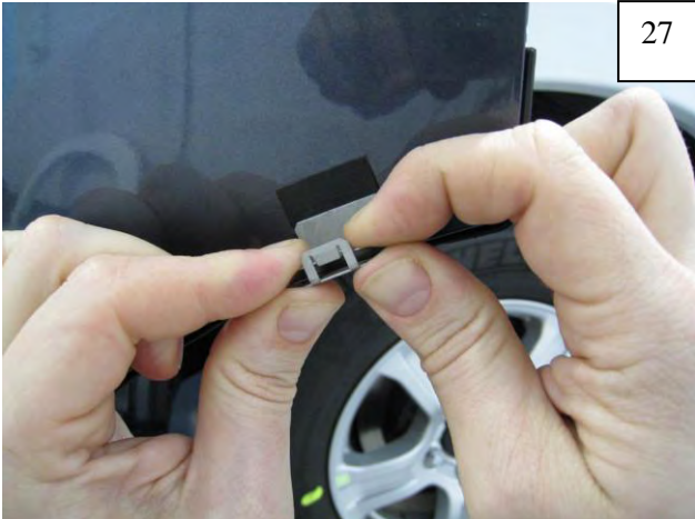
Snap each clip shut once aligned.
