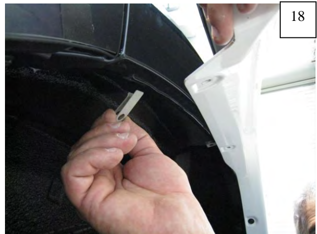
Pull forward portion of flare out from fender gently, and slide two supplied Long Clips onto fender lip, aligning holes in clips with holes in flare.
