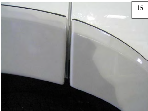
Position Rear Main Flare on fender, aligning with edge of sheet metal along door, but not extending into the door seam.
