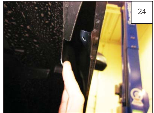
24 Pull wheel well liner out from behind fender lip.
