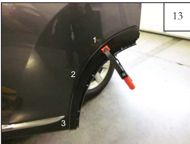
Use the polyfoam as a pad between the inner sheet metal and the ratcheting spring clamp. Attach ratcheting spring clamp on upper part of Inner Door Piece in Position 1 and tighten. Leave clamp in place for at least 1 minute. Repeat clamping Inner Door Piece for positions 2 and 3. Leave clamp in place at least 1 minute in each position.
