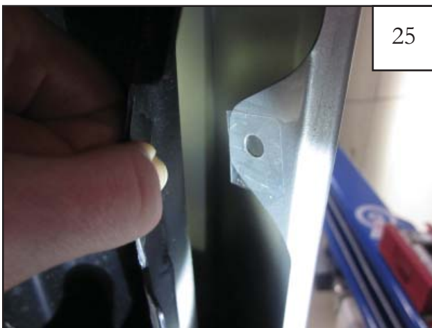
25 Install Tab (MT1-0014) over factory hole locations behind wheel well liner. Reference Step 22 for locations.
