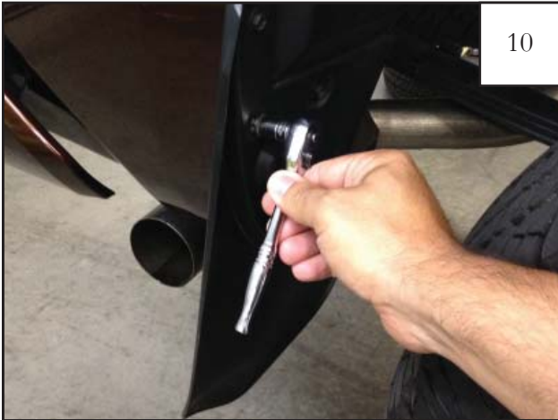
10 Using a socket wrench with a 10mm socket, remove factory screws from the factory mud guard.
