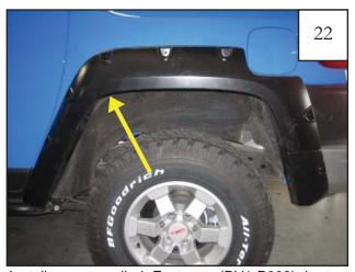
Install one supplied Fastener (RV1-P003) in top forward hole. Check that Edge Trim (GP1-0001) is seated correctly, then tighten all Screws.
