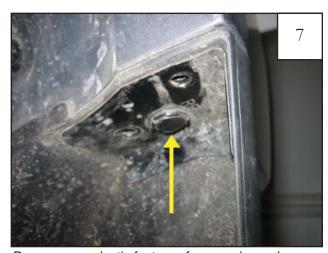
Remove one plastic fastener from mud guard.
