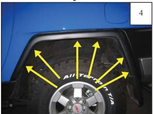
Using a 10mm socket, remove six bolts.
