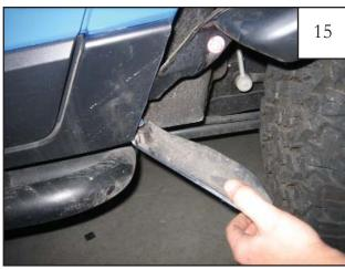
Cut along rocker panel so that it is trimmed flush with sheet metal.
