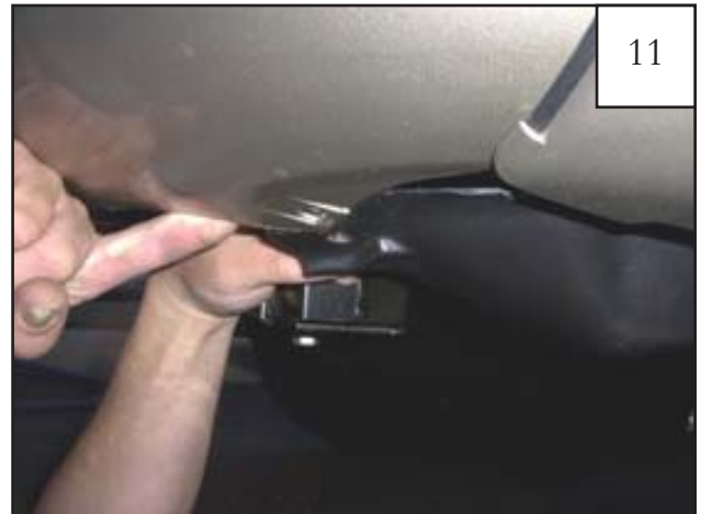
Pull down bumper cover and splash shield.
