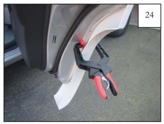
Note: The pressure applied by the clamp or partner may have to be moved from the center so that the plastic is fully set in the clip for the uppermost and lowermost clip locations.
