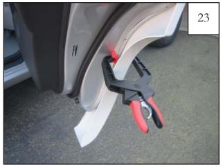
Using either a clamp or a partner, hold door piece in place such that the plastic is fully set in the clip. Starting in the two center locations, tighten screws started in step 22. Once center two screws are installed, tighten the uppermost and lowermost screws.
