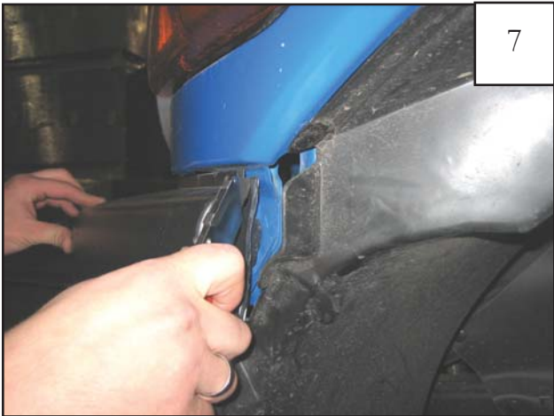
Trim remaining plastic flush with bumper.
