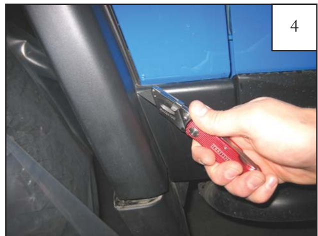
4 Using a utility knife, cut along seam connecting factory flare to rocker. Cut down to mud flap area.
