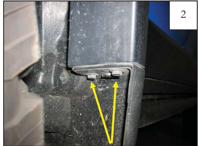
2 Remove two bolts connecting factory flare to mud flap as shown. Note: (1) Factory plastic fastener to be removed in Step 3 is located here as well.
