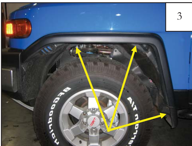
3 Remove three factory plastic fasteners using a flat head screwdriver or pry tool.
