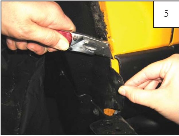
Using a utility knife, cut splash guard flush with edge of a sheet metal.
