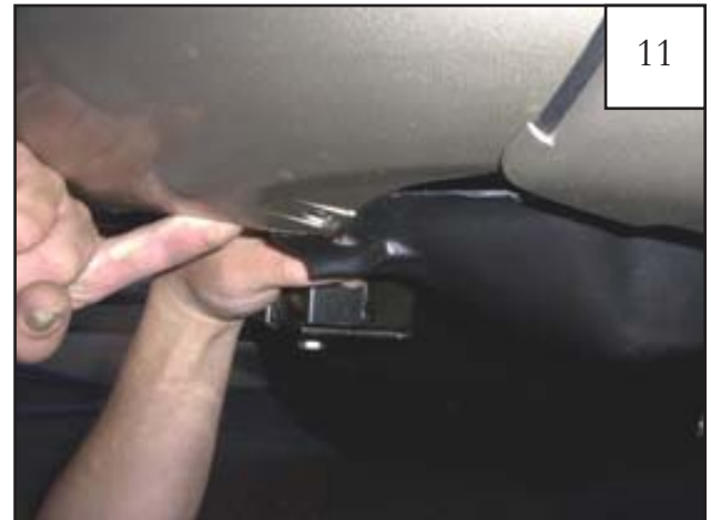
Pull down bumper cover and splash shield.
