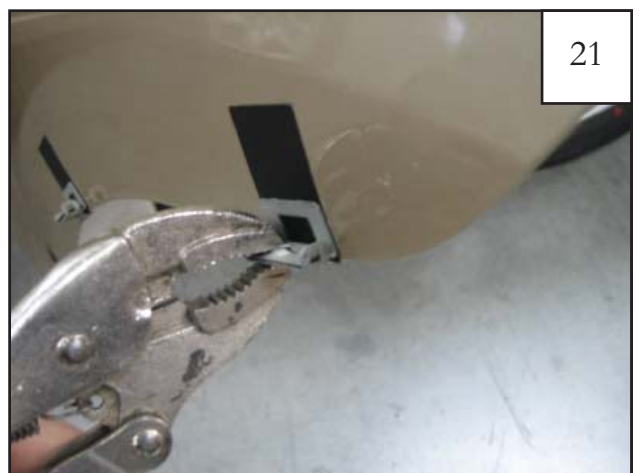
Use vice grips to secure the clip to the sheet metal.
