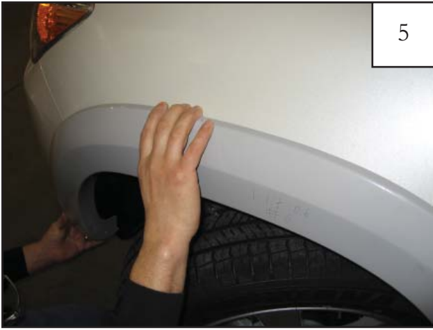
5 Replace flare on fender, aligning holes with the holes in clips.
