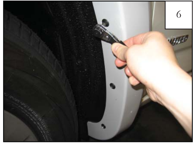
6 Start supplied truss-head screws through three rear holes in flare and into factory holes in rear of wheel well.
