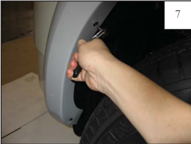
7 Start supplied serrated-flange screws through the three forward holes in flare and into the "S" clips installed in step 4. Using a right angle or stubby Phillips #2 screwdriver, tighten all screws.
