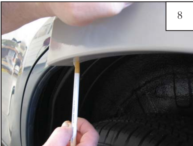
8 Hold the flare firmly on the fender. Using holes in flare as a guide, mark four clip locations with a grease pencil.
