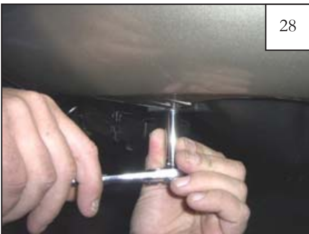
Pull down bumper cover and slide splash shield back in place. Install supplied hex screw(SW1-00036) in front of bumper cover to fasten splash shield to bumper
