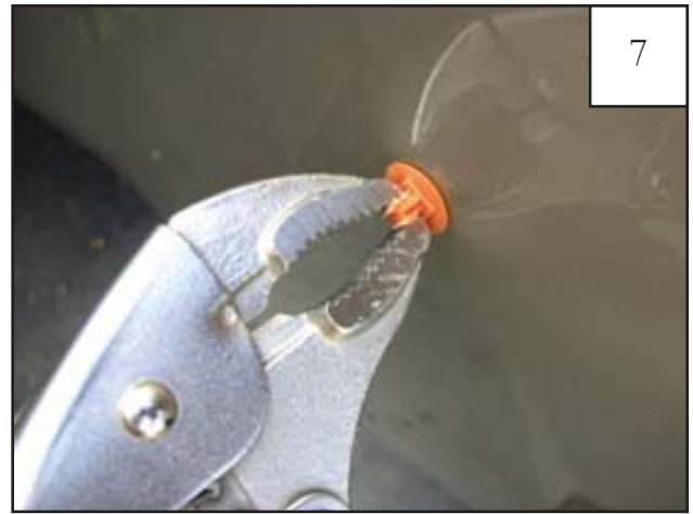
Remove one clip from front using vise grips, pulling with a rocking motion. See step 5.
