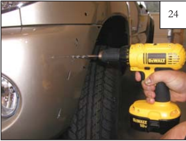
Remove fasteners installed in Step 21-22 and remove flare from fender. Drill at marked places with a 5/16" drill bit
