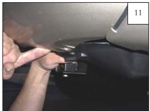
Pull down bumper cover and splash shield.
