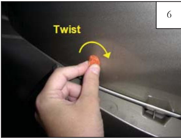
Using a clockwise twisting motion, remove eight factory plastic clips from fender. See step 5.
