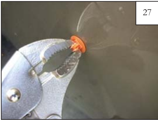
Remove one clip from fender using vise grips, pulling with a rocking motion. See step 28.
