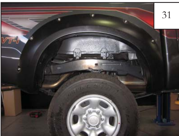
Position flare on fender and re-install factory screws through holes in flare and into factory holes.
