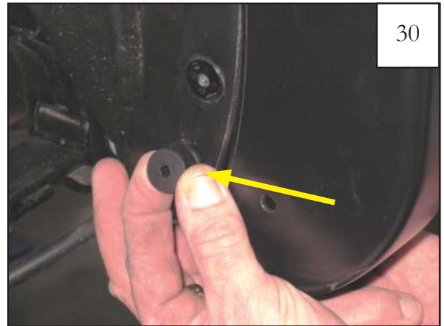
Install supplied grommet (GR1-0001) into factory hole.
