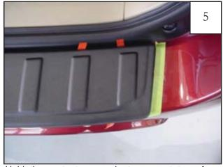
Hold the part at an angle to prevent tape from prematurely sticking, and align the part on the bumper by centering bump in rear door sill between two center ribs in part and using the masking tape applied in Step 2 as a guide.
