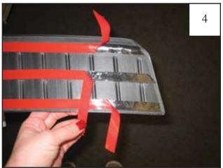
Peel red liner partially from tape pads. NOTE: Make sure tabs are folded toward the outside of the part and that the middle tape liner is in front of rear liner.
