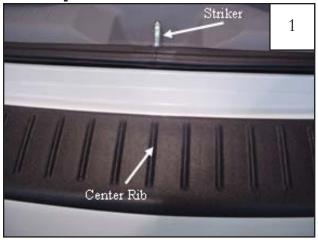
Open rear door of vehicle. WITHOUT peeling liner from tape pads, align part on bumper, centering the center rib of the bumper guard with metal loop on striker.
