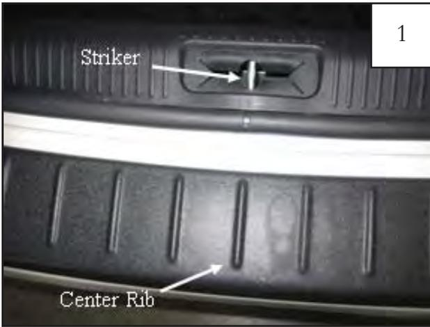
Open rear door of vehicle. WITHOUT peeling liner from tape pads, align part on bumper, centering the center rib of the bumper guard with metal loop on striker.
