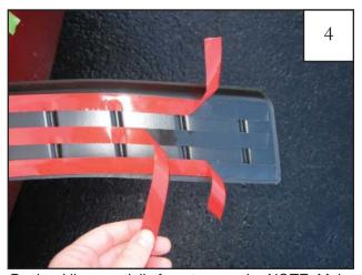
Peel red liner partially from tape pads. NOTE: Make sure tabs are folded toward the outside of the part and that the middle tape liner is in front of rear liner.
