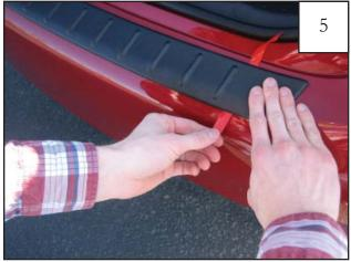
Hold the part at an angle to prevent tape from prematurely sticking and align the part on bumper by aligning shorter center rib in part with center of striker latch location and using the masking tape applied in Step 2 as a guide. Stick peeled end to Bumper and pull tab nearest the rear of the vehicle while applying downward/forward pressure to the rear edge
