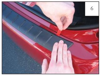
Maintaining part placement, repeat process for center liner closest to center of vehicle.
