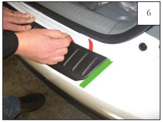
Maintaining part placement, stick peeled end to bumper and pull tab nearest the rear of the vehicle while applying downward pressure to rear edge of part. Repeat process for liner for center tape, then liner towards the front of the vehicle.
