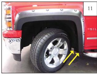
Locate flare into position on vehicle. Install supplied screw (SW1-0056) through two bottom rear holes in flare and into factory hole in rear of wheel well.
