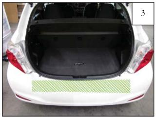
Make sure that all installation surfaces are free of dirt and/or grease. Use a clean, lint-free cloth and isopropyl alcohol-based cleaner.
