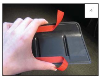
Peel red liner partially from tape pads. NOTE: Make sure tabs are folded toward the outside of the part.
