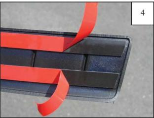
Peel red liners partially from tape pads and fold towards outside of part.
