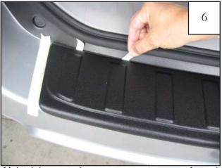
Maintaining part placement, repeat process for red tab liner nearest the front of the vehicle.
