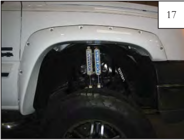
Completed front flare installation.
