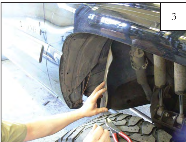
Pull splash shield forward out of the way.
